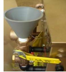
Then charge the generator with clean water. Pour water through the funnel until the sight-glass shows nearly full. Then close the yellow gate valve. Dry the surroundings. **Note:** if the unit has not been used for a while, **flush out the tank repeatedly.** Do this about every month too. Use the bottom (blue) drain valve for this. Shake the unit about to slosh junk from the bottom of tank!
