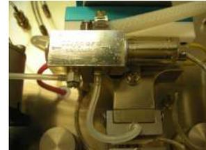
Now connect the pilot actuator lines (small diameter clear tubing fixed to the round actuator cylinders at the rear of the dosing valves) to the two air ports formerly used to provide air for the bond cooling head. Ensure that the connectors are fully screwed down (they can be stiff).
