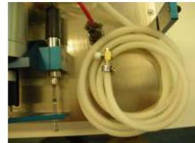
Unwind the soft neoprene tube and lay it so it hangs over the side of a water container (pointing away from ABES and the operator). Steam (and initially water) will come out of this when the system is running.
