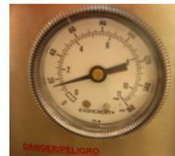
rotating it a small amount (maybe 1/8 turn) in or out as appropriate (clockwise to increase pressure and anti-clockwise to reduce it). Repeat this procedure again if necessary until the “switch-off” pressure lies between 15 and 20psi.
